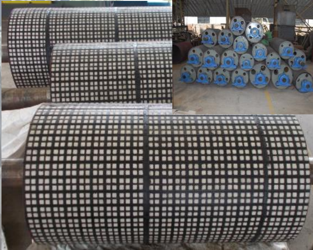
Pulley lagged with Ceramic Tiles
